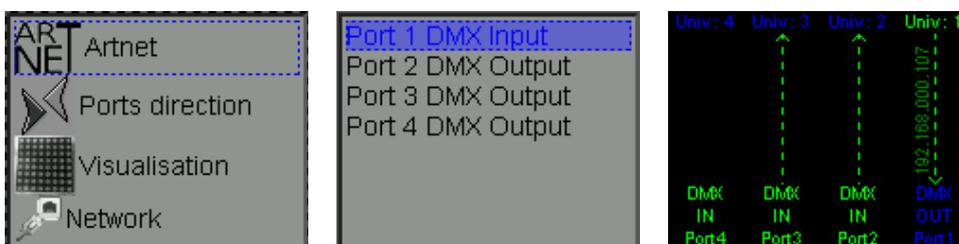
The DMX4-E-gate is provided with 4 DMX ports, which are converted to the ArtNet protocol; both from ArtNet to DMX and vice versa. In order to do this we can configure DMX ports in the gate as input or outputs. This function is visualised on the main screen, where both the direction of the data flow and the ID number of a controller to which or from which data are transferred are shown.
