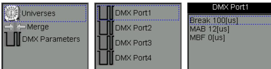
On account of the diversity of devices on the market and sometimes the lack of conformity to the standard the DMX512 - E-Gate is provided with a function of changing the output DMX parameters. Options allow to select proper output signal parameters for a given device.
