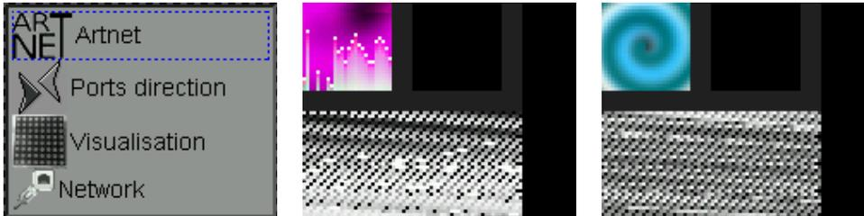
The DMX4-E-gate is provided with a very useful function (visualization), which enables monitoring on the screen data, which are sent with the ArtNet protocol. This monitoring is possible both in the RGB and Mono mode. Visualisation parameters can be changed in the “Patching visual” submenu.
