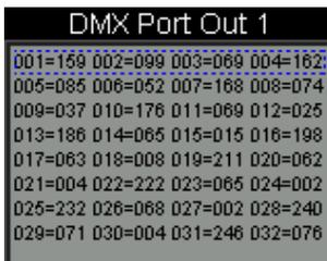
DMX Port Out x. Basing on this we can watch the output or input DMX values depending on the port direction, which is set according to the ART-Net protocole.
