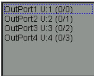
In this submenu we can ascribe a right Univers to a DMX port. To do this we select an appropriate output OutPort pushing the up- or down-arrow and we push down (click) the joystick - a Port will be highlighted. Pressing the joystick up or down you select an appropriate Univers number. Next, you have to pres (click) the joystick again. The values will be saved.
