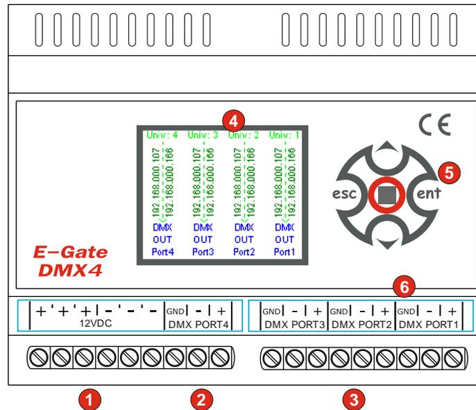
1. Power supply joint (+12V, GND)
