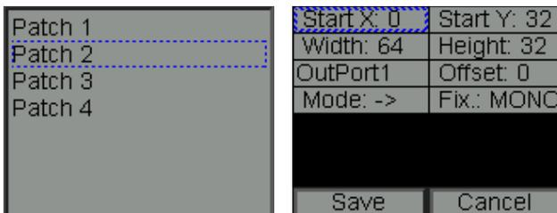
The gate is provided with a very easy to use function of monitoring data from ArtNet in the form of pixels displayed on the screen. You have 2 modes you can use: Mono, which occupies the first channel and RGB occupying three channels. The screen can be divided into 4 parts (Patch 1-4) and each of these can be properly placed on the display. You can change the following parameters:
